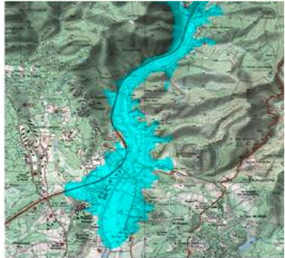
Flood Inundation due to Malpasset Dam-Break Event Simulated by NCCH Flood Simulation System
